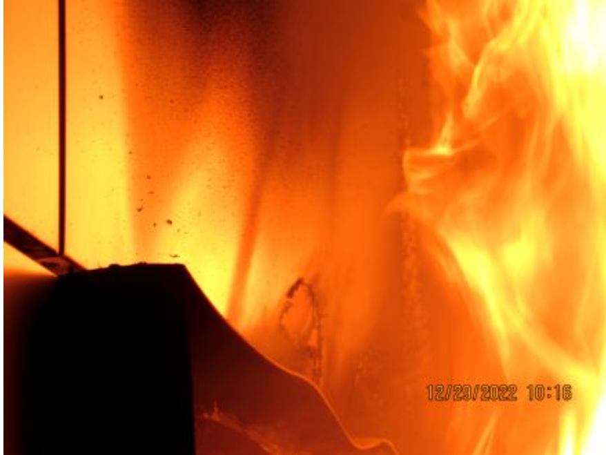
Photo No. 17 Panels above opening beginning to open up
