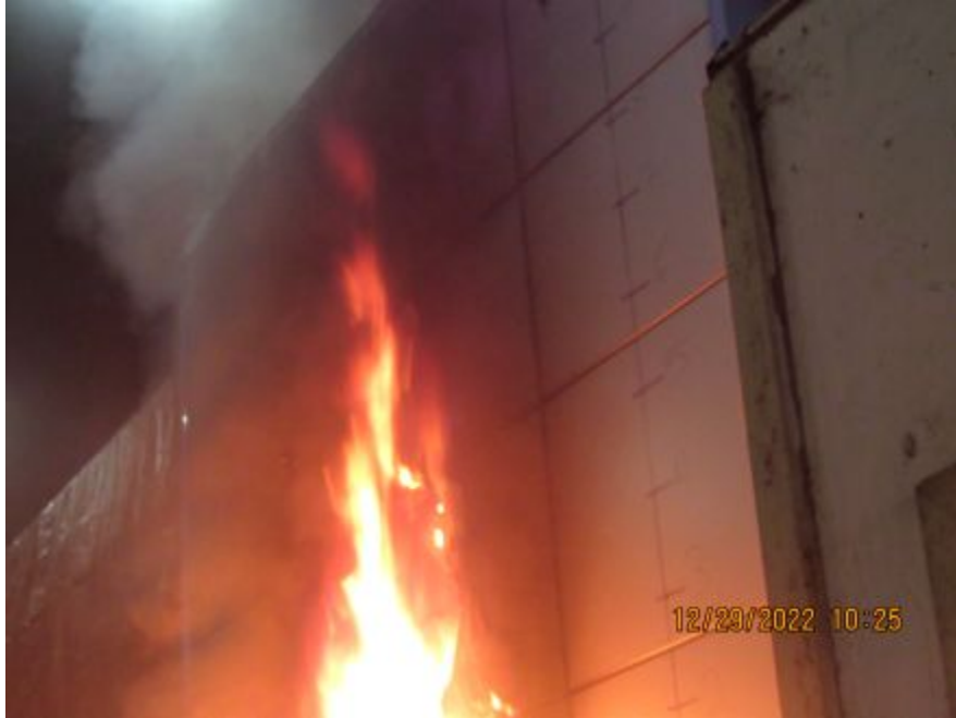
Photo No. 19 Flaming on sample at 5.5 feet
