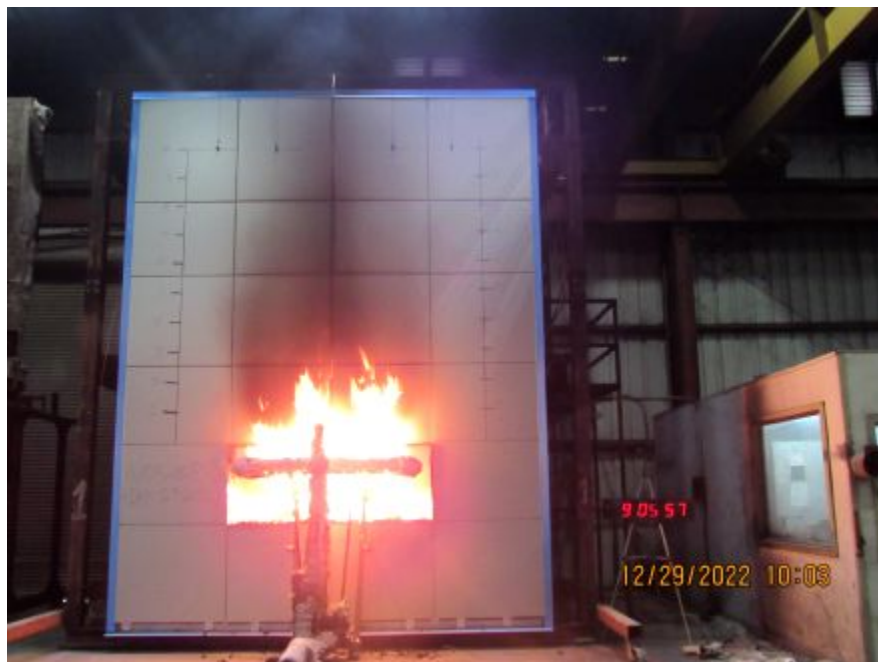
Photo No. 16 Window burner ignited
