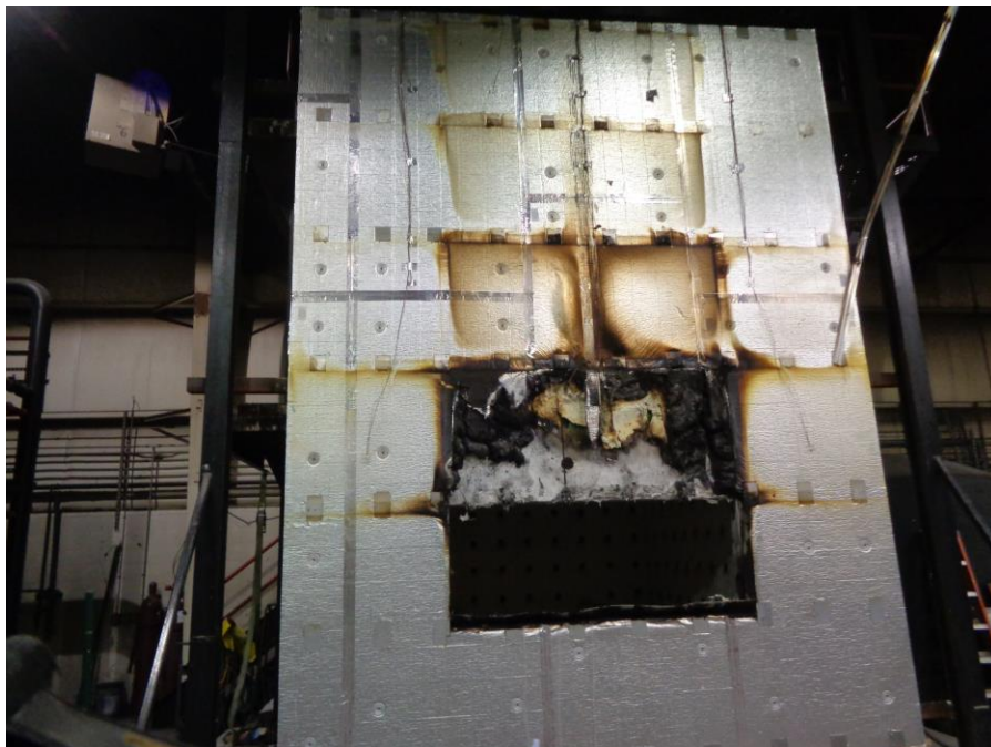
Photo No. 14 Exterior Cladding Removed & Burn Pattern of Insulation (Post-test)
