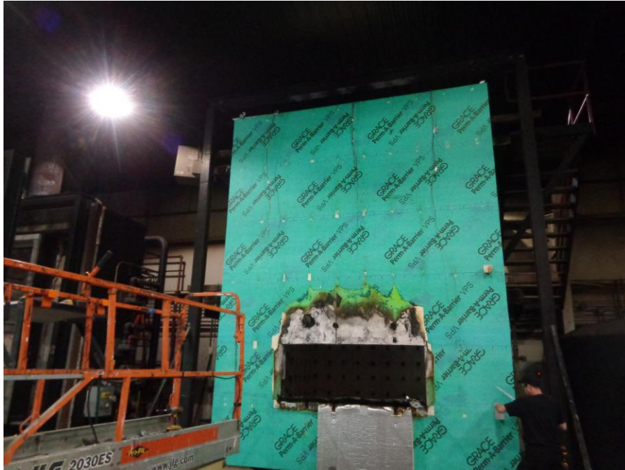
Photo No. 15 Exterior Insulation Removed & Burn Pattern of AV Barrier (Post-test)
