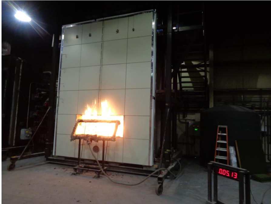
Photo No. 9 Ignition of the Window Opening Burner
