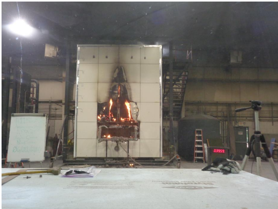
Photo No. 12 Exterior Cladding Burn Pattern (Post-test)
