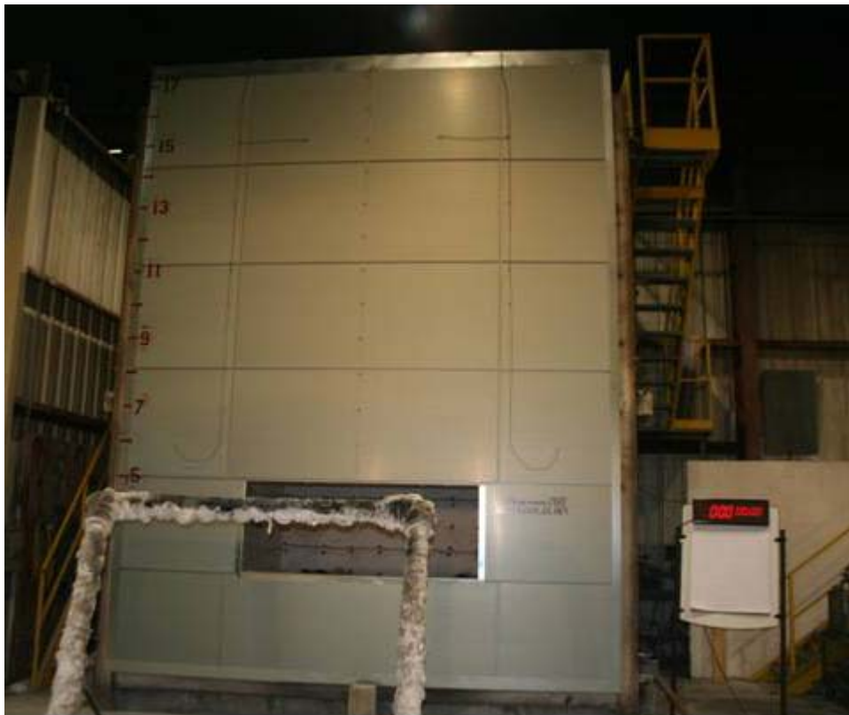
Figure B-2. Completed Wall Assembly prior to Test.
