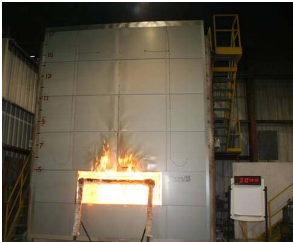
Figure B-6. Exterior View of Wall Assembly at 10 min 49 s into Test.
