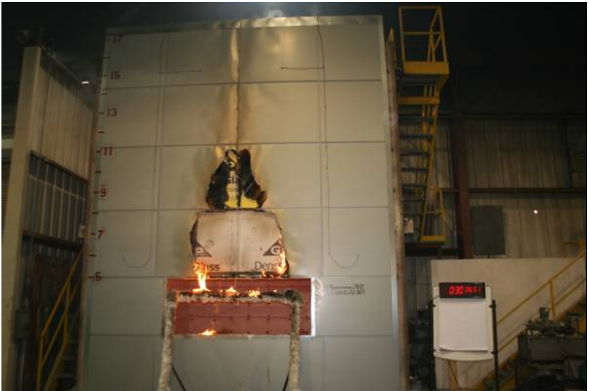
Figure B-12. Exterior View of Wall Assembly at End of Test.
