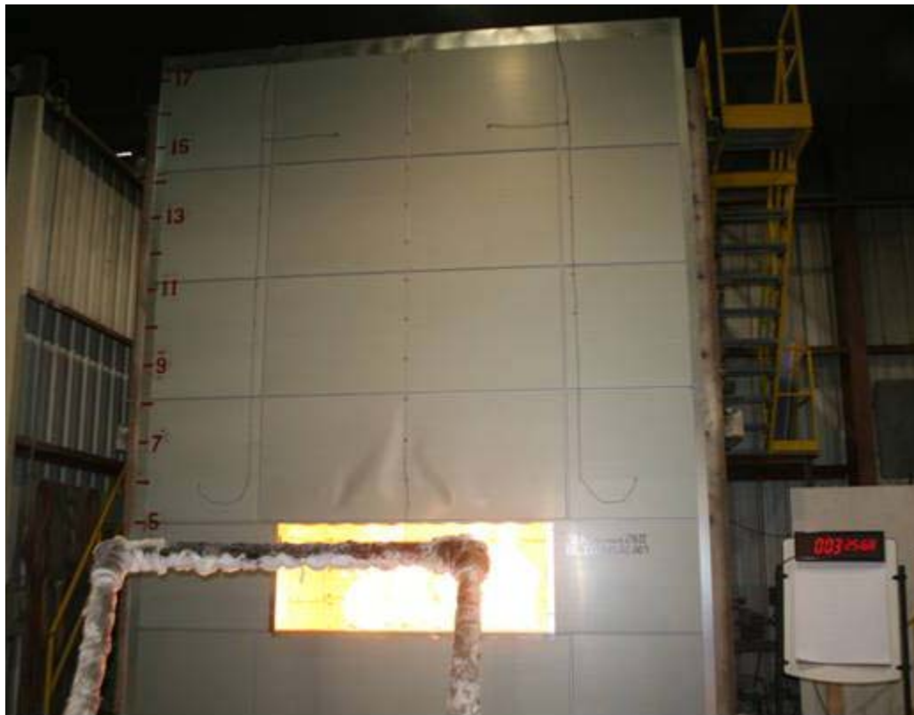
Figure B-4. Exterior View of Wall Assembly at 3 min 25 s. Warping of Exterior Panel Skin Visible.
