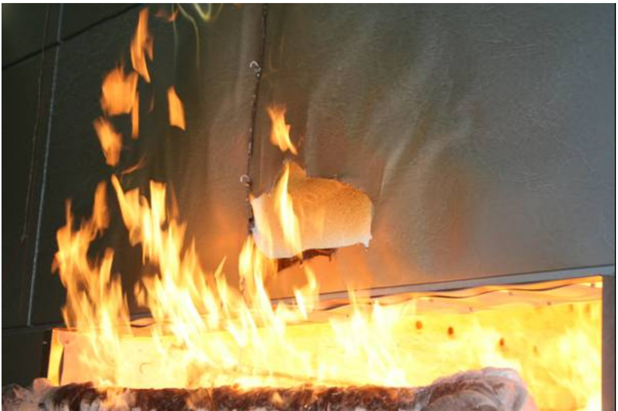
Figure B-8. Opening of Exterior Panel Skin at approximately 11 min into Test.
