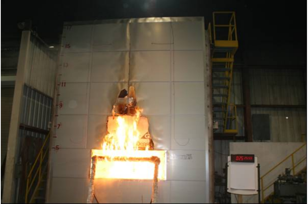
Figure B-11. Exterior View of Wall Assembly at 25 min 25 s into Test.
