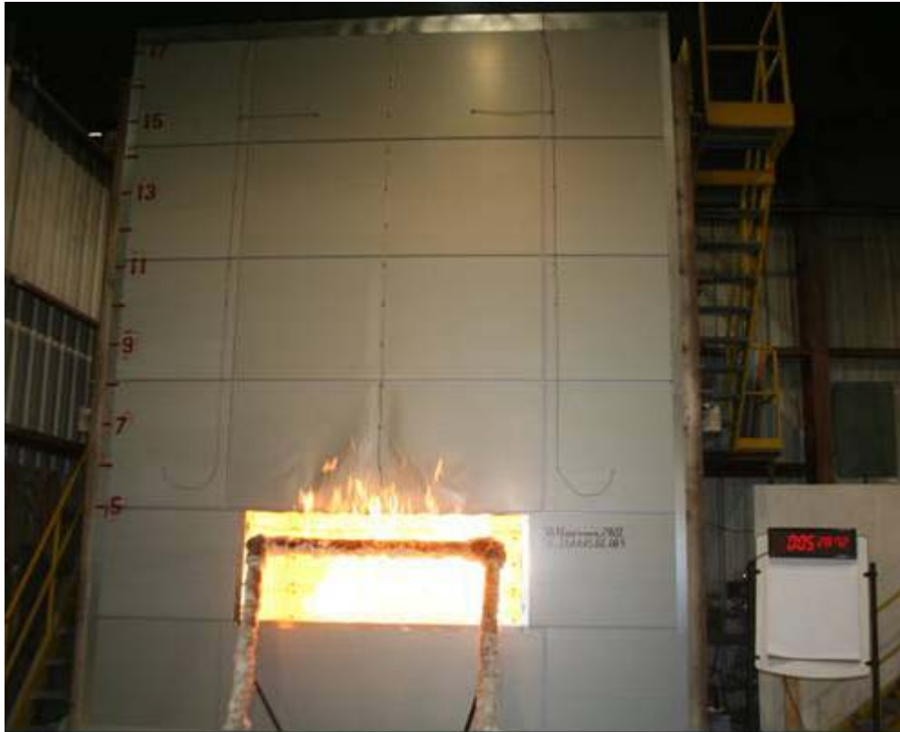
Figure B-5. Application of Window Burner at 5 min.
