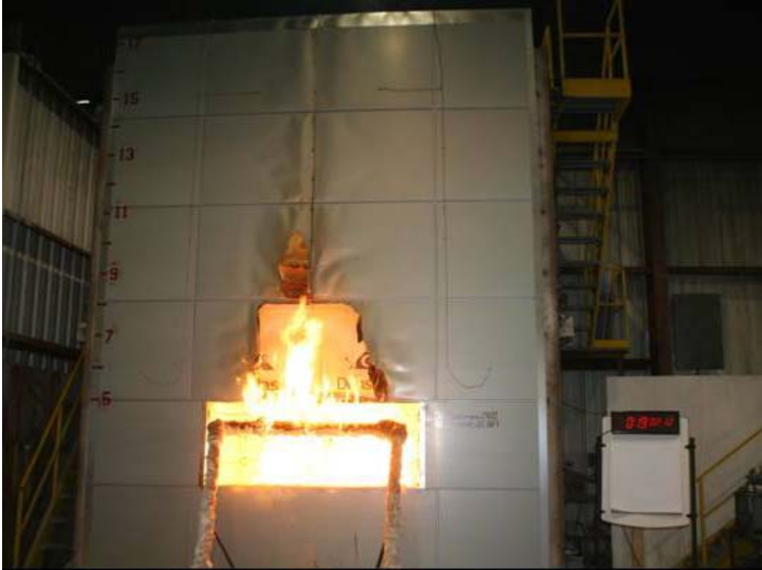
Figure B-9. Exterior View of Wall Assembly at 19 min 2 s into Test.
