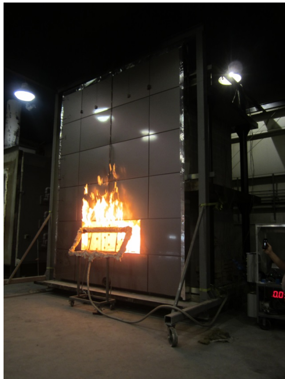
Photo No. 14 Ignition of Window Opening Burner www.archtest.com
